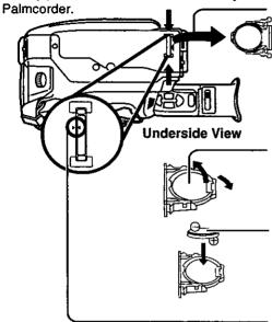
I While pinching the stopper tabs, pull the tray out of the Battery Compartment.
