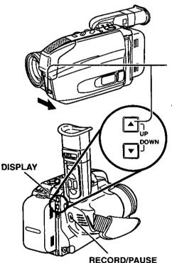
I While pressing the UP ▲ button, set the POWER switch to CAMERA.
