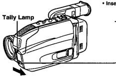
Set the POWER switch to CAMERA. Built-In Lens Cover opens. **EVF**
