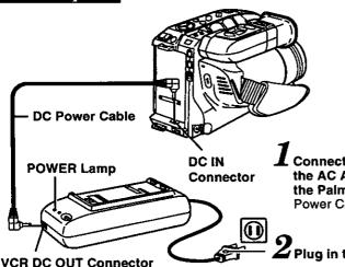
Connect the VCR DC OUT on the AC Adaptor to the DC IN on the Palmcorder with the DC Power Cable (supplied).
