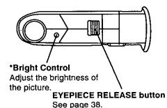
\*Note: These controls have been set at the factory. It is not necessary to adjust these controls under normal circumstances. But, should it become necessary, be careful to make the adjustment with a small, slender screwdriver so as not to damage the miniature control.
